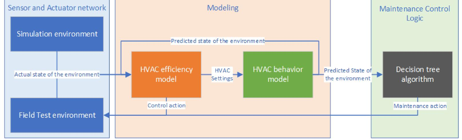
The system operates with two control loops: 1) energy efficiency is managed by the HVAC optimization model, and 2) preventive maintenance is governed by a decision tree algorithm, based on predictions from the HVAC behavior model.
