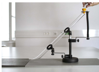
Images: The pattern of scattered material shows the slip resistance class of the floor (left). Prototype of the TU Wien floor slip tester with a height of about 20 cm (right).
