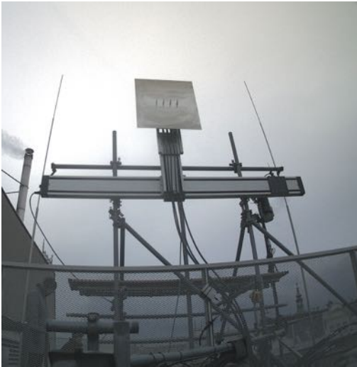
Virtual full-dimension MIMO measurement test-bed.
