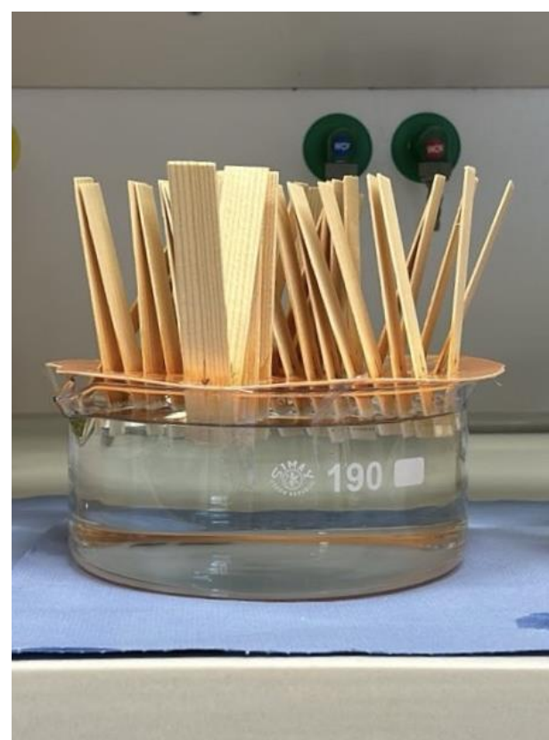
Delignification of veneers with peracetic acid
