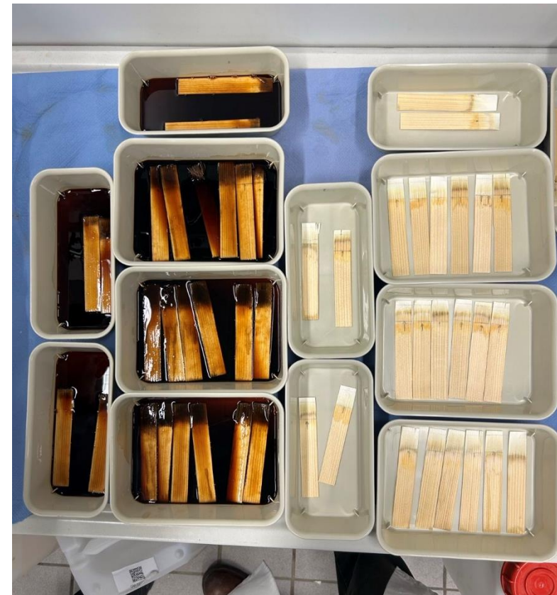
Impregnation of treated veneers with lignin supernatant
